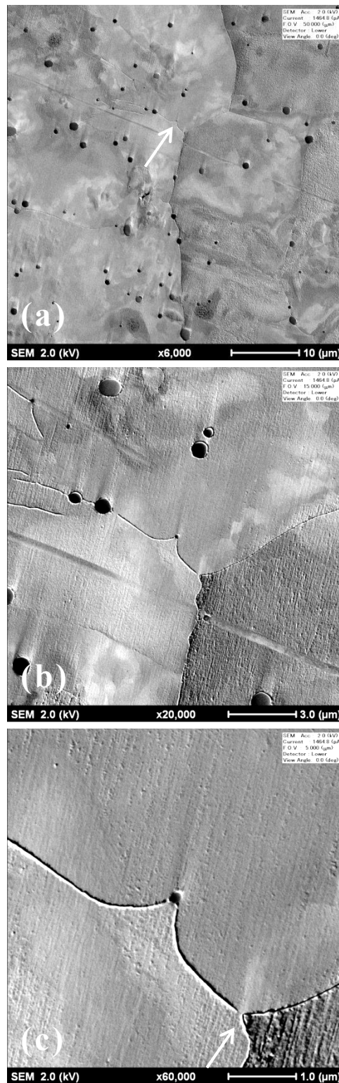
Fig. 2-8 FE-SEM micrograph of Base annealed at 900°C for 21.6 ks. Grain boundaries were pinned by Cr precipitates to suppress boundary migration.
