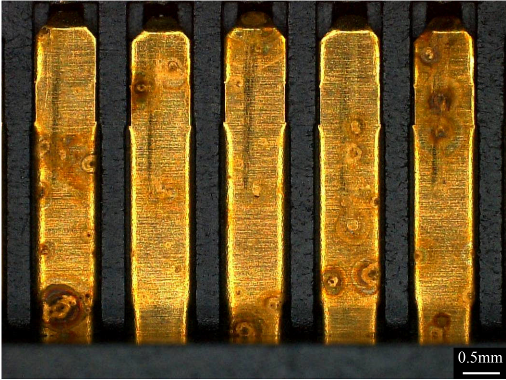
Fig.5-1-7 Result of sealing (soluble) /Au (0.8 \mu m)/Ni-P/Brass samples after four mixed gas flow corrosion resistance test by S-ATA standard.
