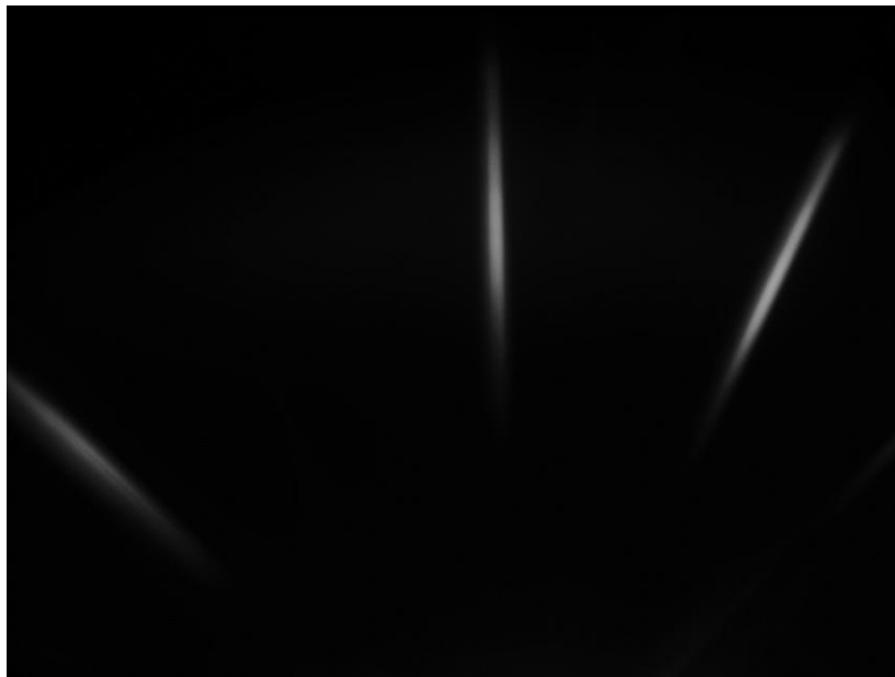
Fig 4.9 spectrum obtained in CCD after focusing on a 40mm achromatic lens.
