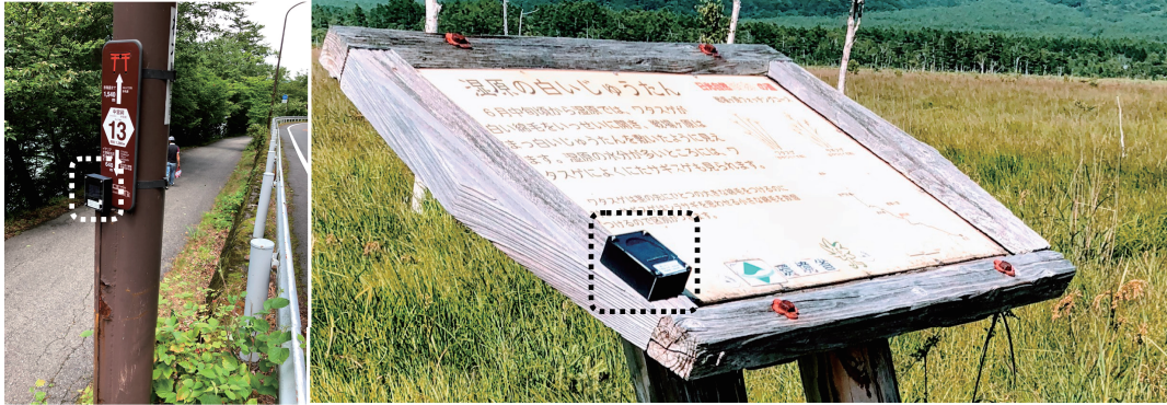
Fig. 4.6: Installed Solar BLE Beacon in Oku-Nikko
