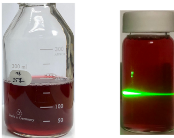
Fig-2.2 Tyndall effect created by the prepared AMIET-AuNPs
