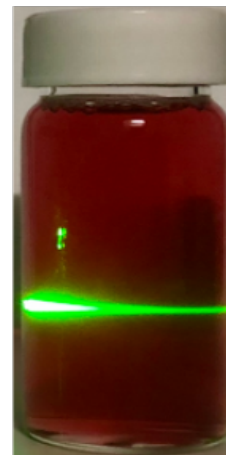
Fig-1.4 Light scattering by colloidal gold
