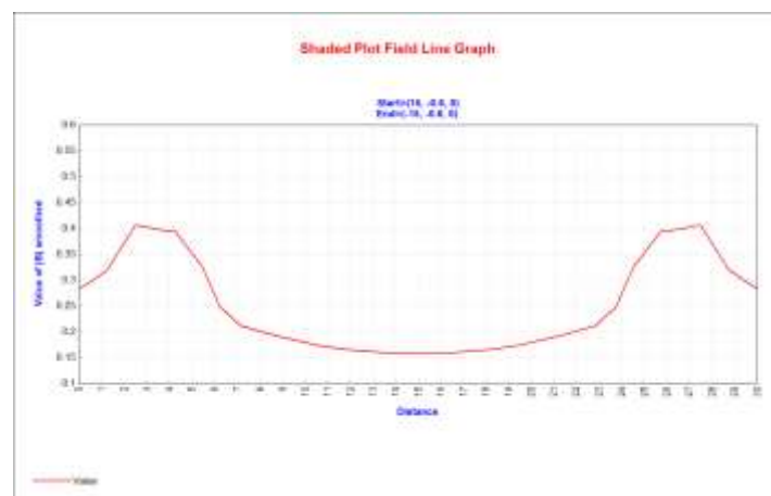
(c) Magnetic field intensity curve at 0.5mm from the magnetic pole
