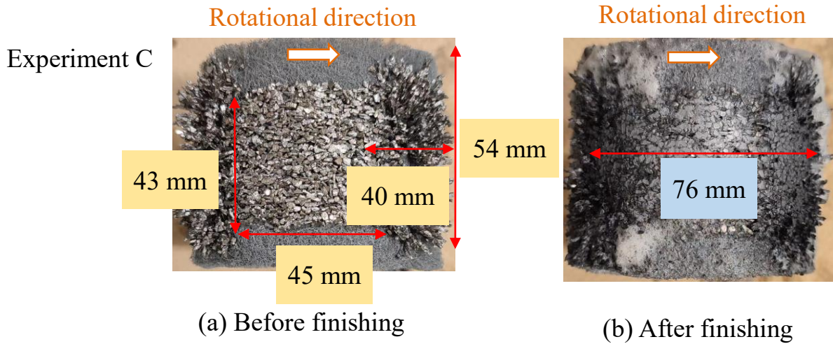
Fig.5.10 Photographs of magnetic machining tool before and after finishing
